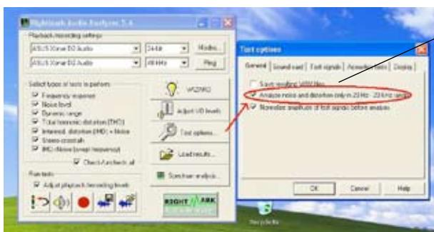
4. Go to the Sound Card tab and select “DirectSound” as the Driver Model (because Windows MME mode doesn’t support high-resolution 24bit and 192KHz audio playback.)
