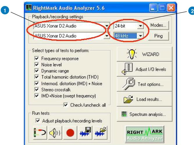
3. Click “Test options” button in RMAA and check “Analyze noise and distortion only in 20Hz-20KHz range” (audio in-band for human hearing) in the General tab.
