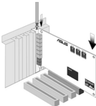
2. Secure the audio card bracket to the back of your computer with the screw that you removed. Refer to section 3.1.
