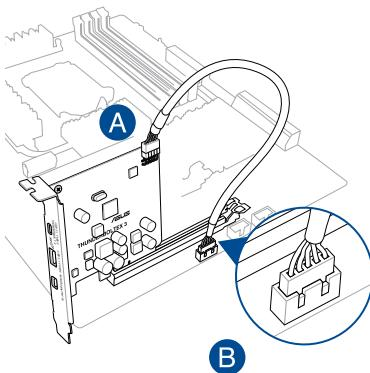
5. Connect the DisplayPort cable to the ThunderboltEX 3 card's Mini DisplayPort IN port (A) and to the DisplayPort on the motherboard's I/O port (B).
