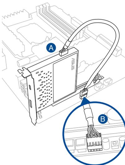
5. Connect the DisplayPort cable to the ThunderboltEX II card's DisplayPort IN port (A) and to the DisplayPort or mini DisplayPort on the motherboard's I/O port (B).
